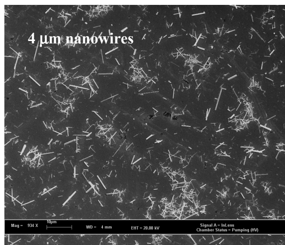
Figure 4.1.b. SEM images of aggregates of “single” \text{WO}_3 nanowires after 5 minutes, 20 minutes, and 1 hour of ultrasonication (10, 6, and 4 \mu\text{m} average length, respectively).
